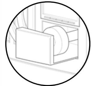
The tape roll access door allows easy changing of tape rolls.
